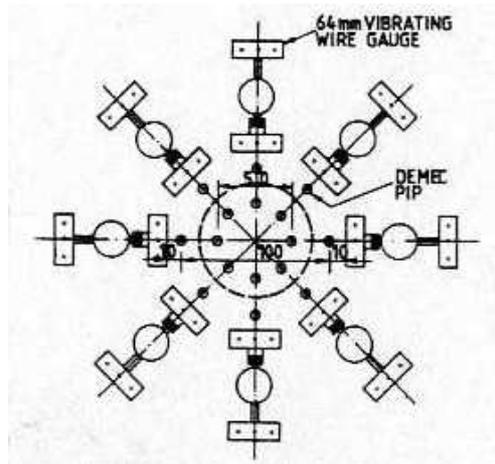
Figure 1 Gauge arrangement for the 75mm diameter cores
