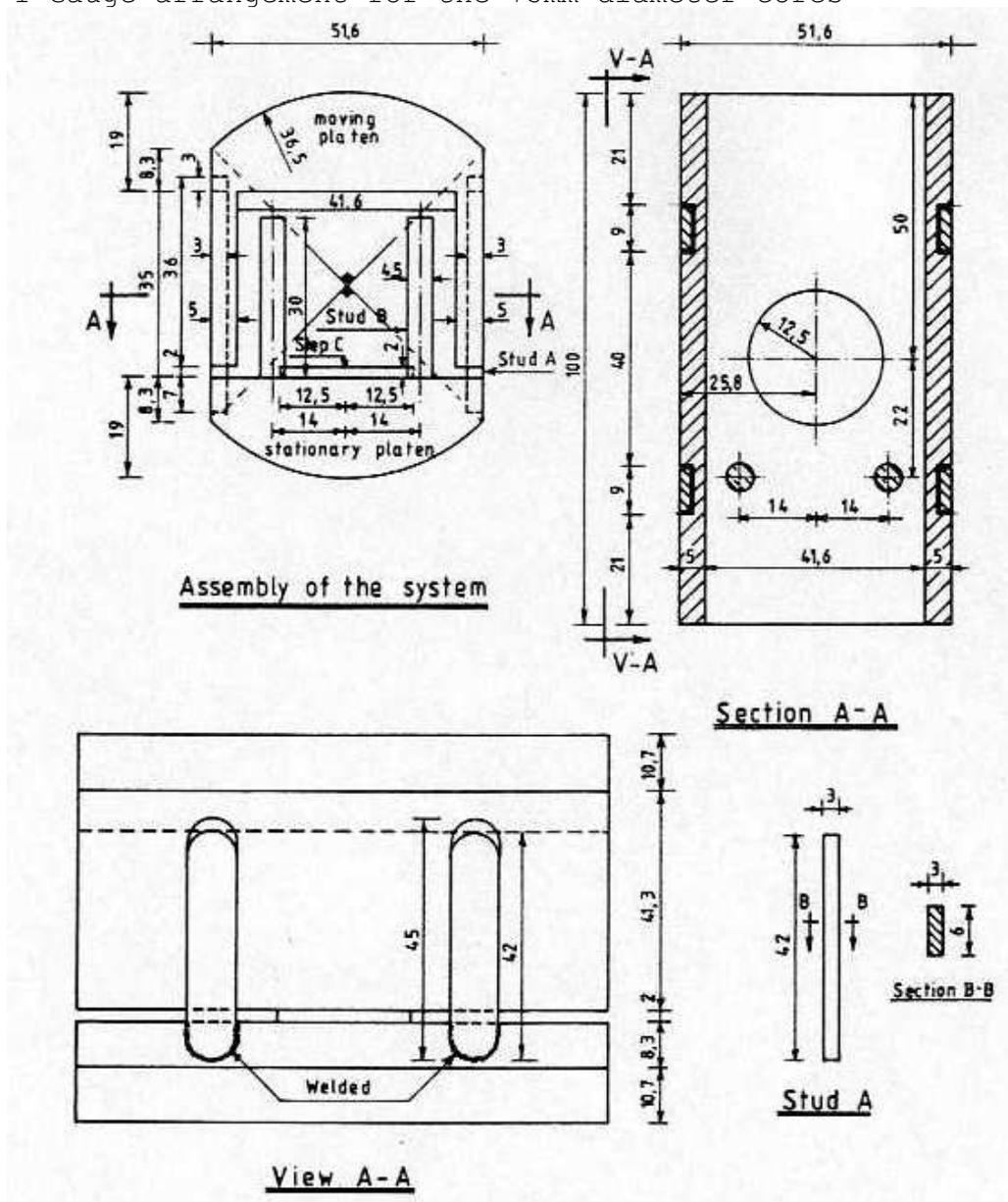
Figure 2 Jacking assembly for 75mm Diameter holes
