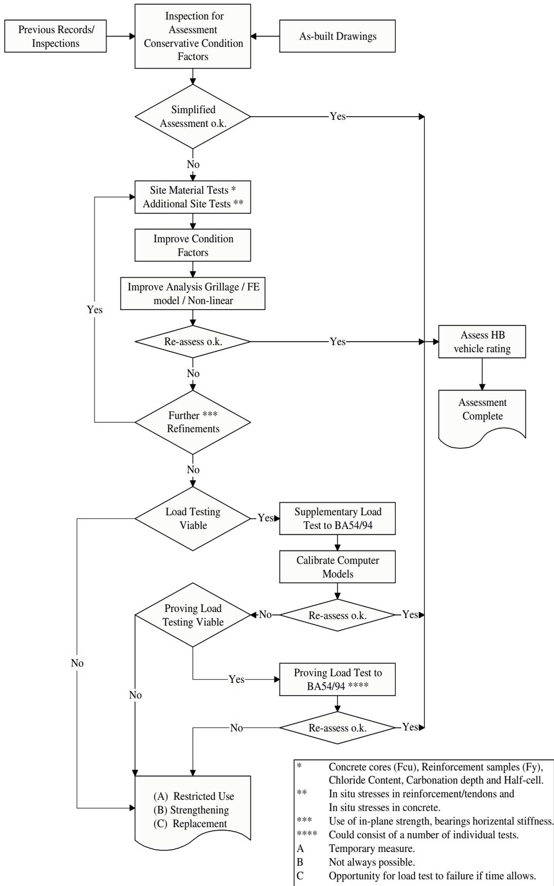
Figure 1. Flowchart of Bridge Assessment including Load Tests
